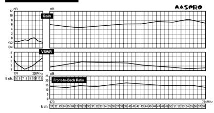
All graphs are produced using MASPRO's original, fullyautomatic antenna measuring device.
